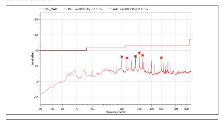
Site: **Antenna: Horizontal Temperature**(C):23(C) **Humidity(%):57%** Limit: FCC Part 15 C 3m Radiation(QP)
