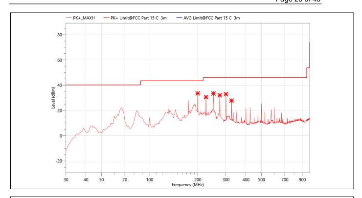
Site: **Antenna: Vertical** Temperature(C):23(C) Limit: FCC Part 15 C 3m Radiation(QP) **Humidity(%):57%**
