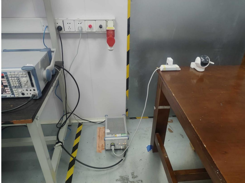
Conducted emissions at AC power line (150kHz-30MHz)
