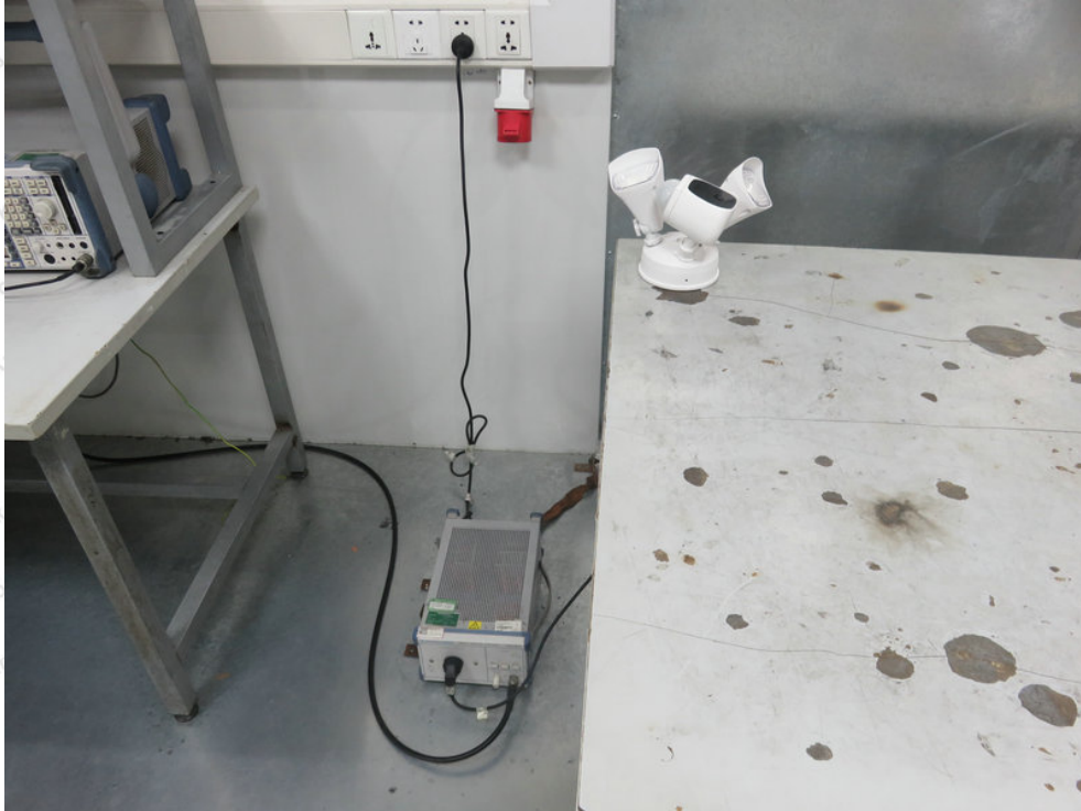
Photo of Power Line Conducted Emission Test
