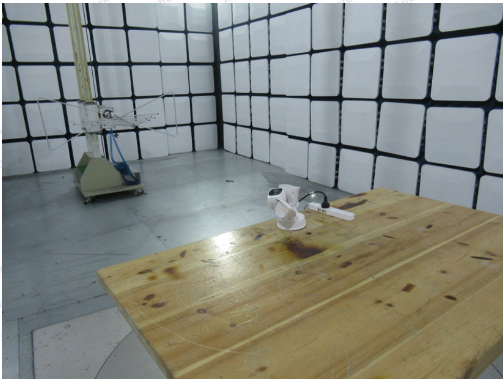
Photo of Radiation Emission Test
