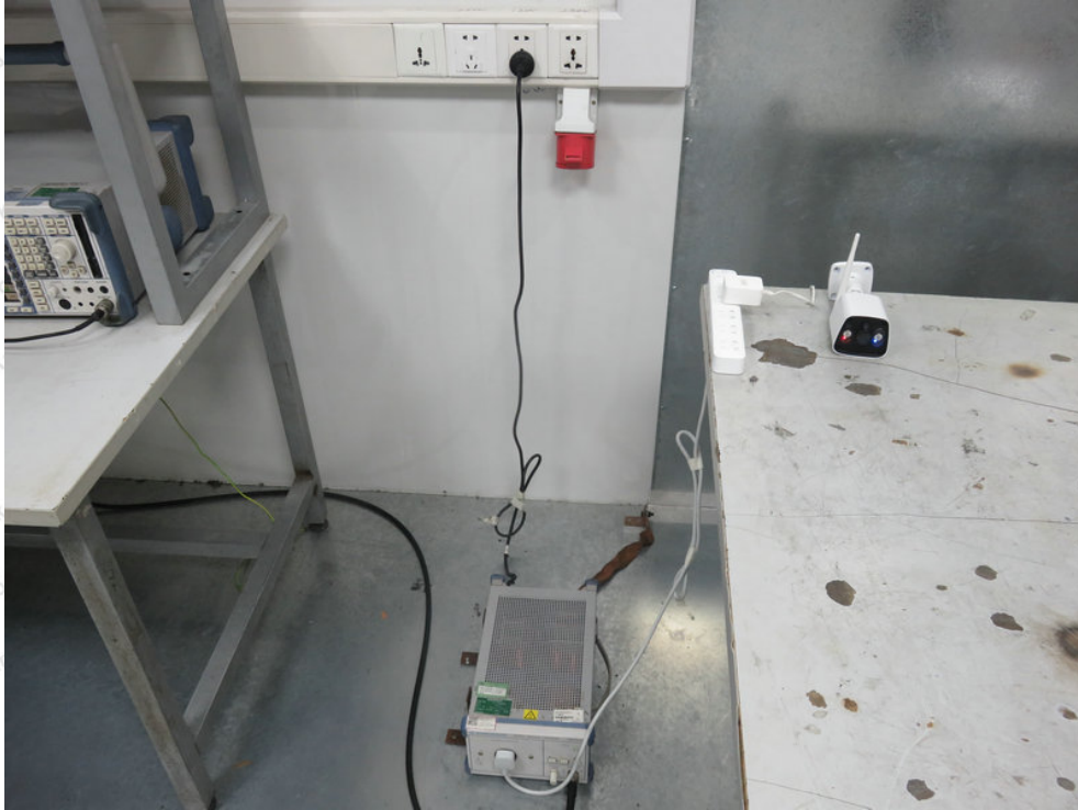
Photo of Power Line Conducted Emission Test
