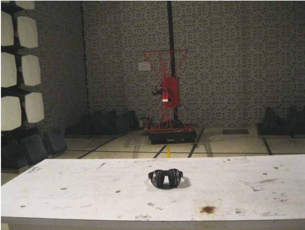
TEST SETUP OF RADIATED EMISSION (30MHz-1GHz)
