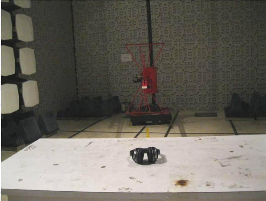
TEST SETUP OF RADIATED EMISSION (30MHz-1GHz)
