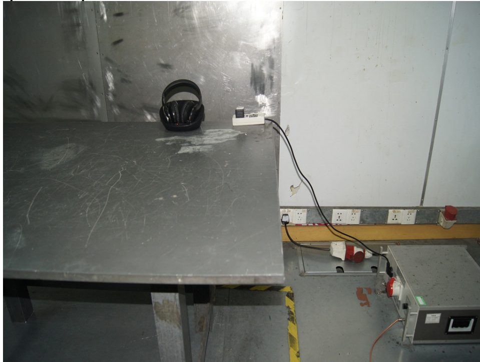
Photograph 2: Set-up for Radiated Emissions
