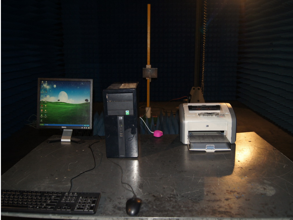
Photograph 7: Set-up for Radiated Emissions, above 1GHz
