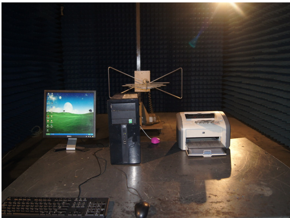
Photograph 6: Set-up for Radiated Emissions, below 1GHz
