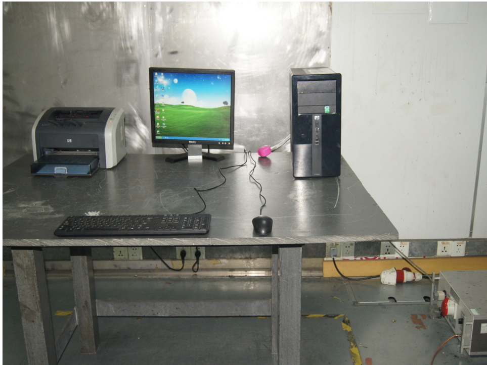
Photograph 6: Set-up for Radiated Emissions, below 1GHz
