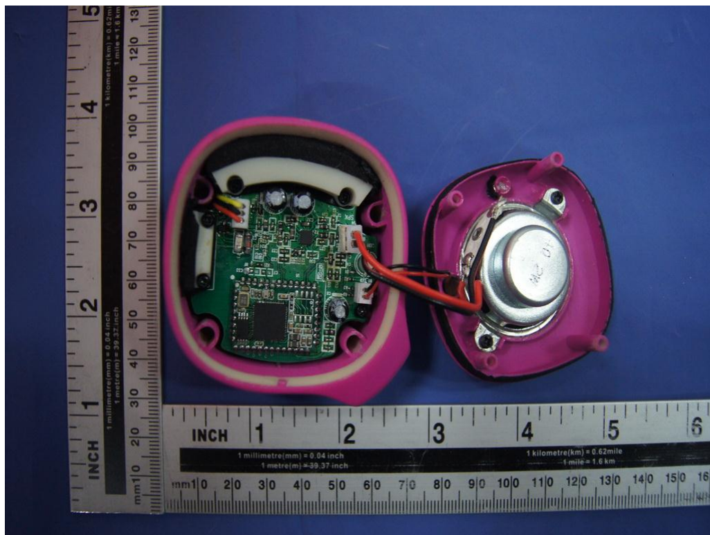
Fig. 8: Internal view of NS-CSPBT03
