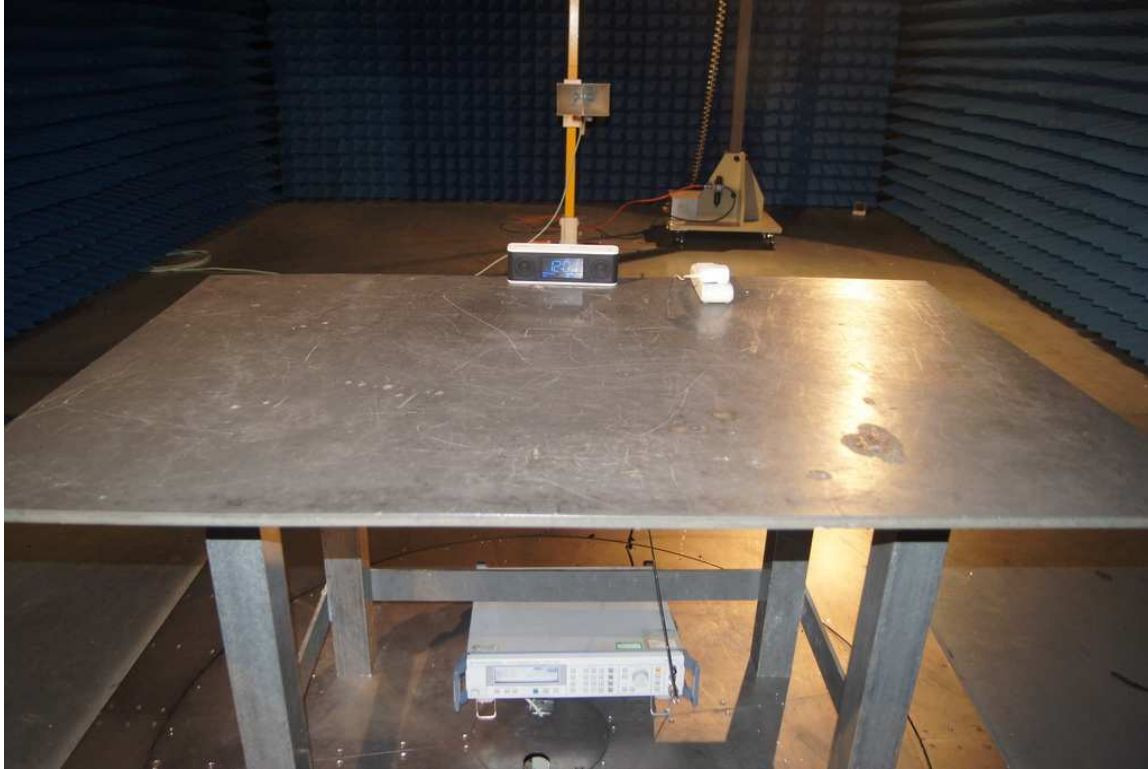
Photograph 7: Set-up for Radiated Emissions, above 1GHz
