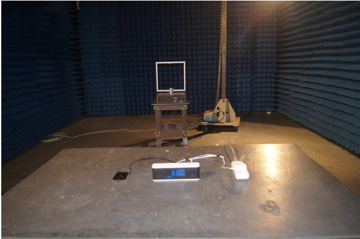
Photograph 2: Set-up for Spurious Emissions (30MHz-1GHz)
