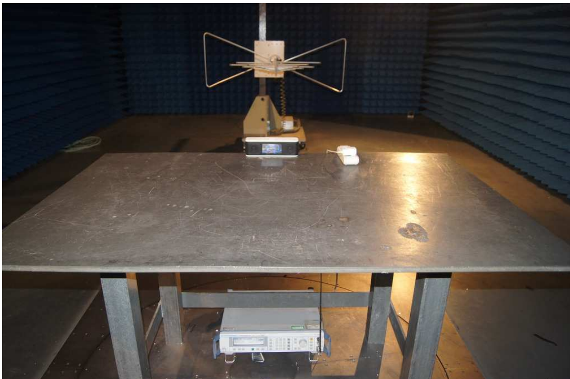
Photograph 6: Set-up for Radiated Emissions, below 1GHz
