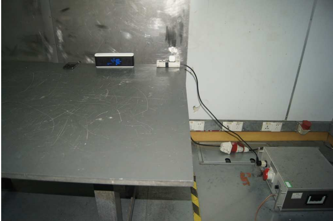
Photograph 6: Set-up for Radiated Emissions, below 1GHz
