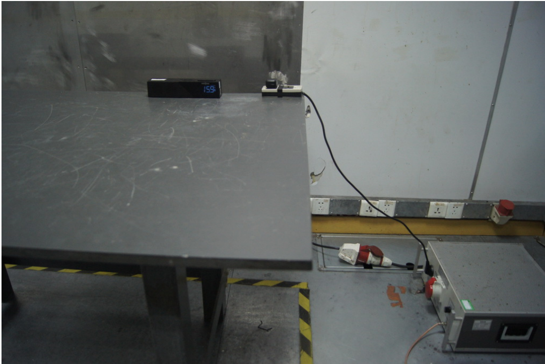
Photograph 6: Set-up for Radiated Emissions, below 1GHz
