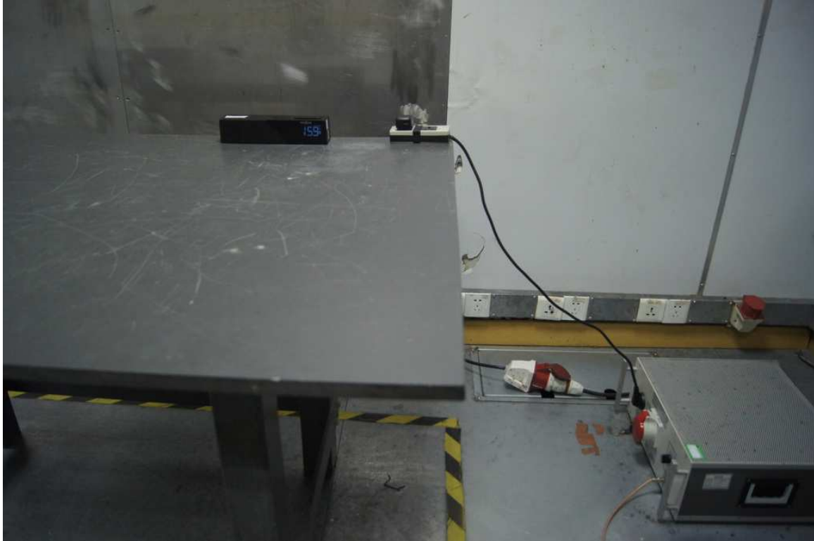
Photograph 6: Set-up for Radiated Emissions, below 1GHz
