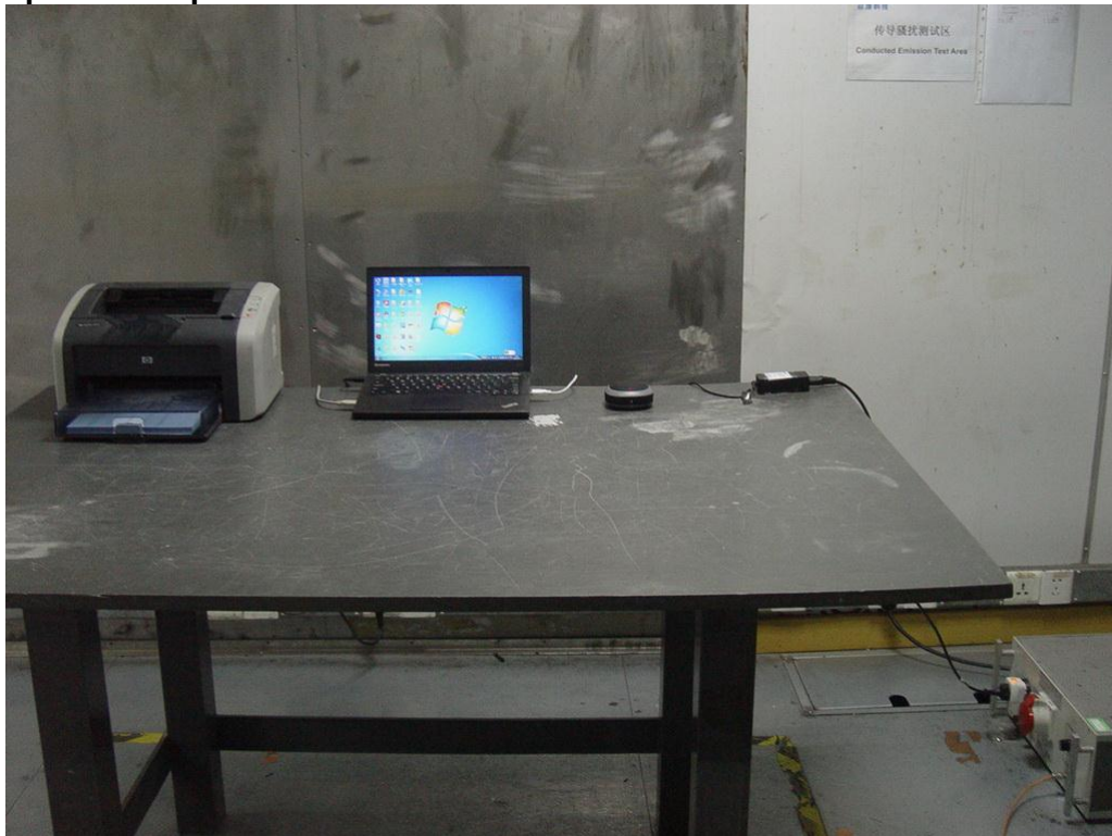
Photograph 2: Set-up for Radiated Emission of below 1GHz
