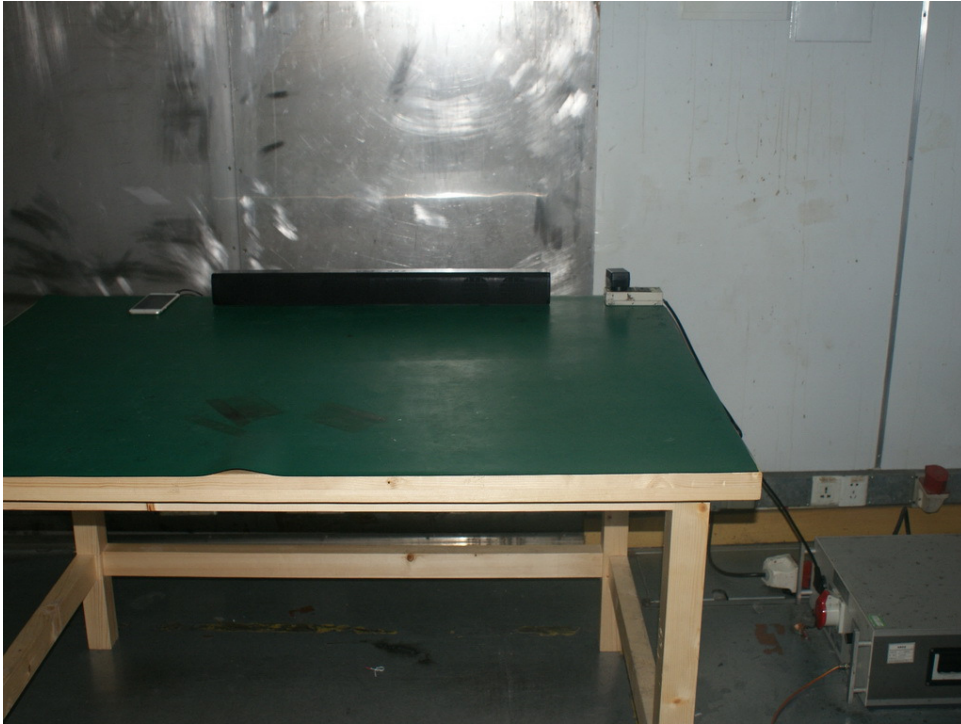
Photograph 6: Set-up for Radiated Emissions, below 1GHz
