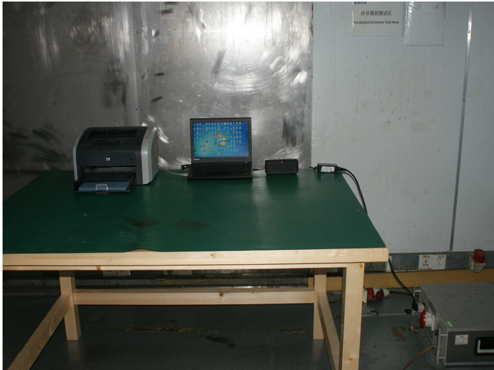
Photograph 6: Set-up for Radiated Emissions, below 1GHz
