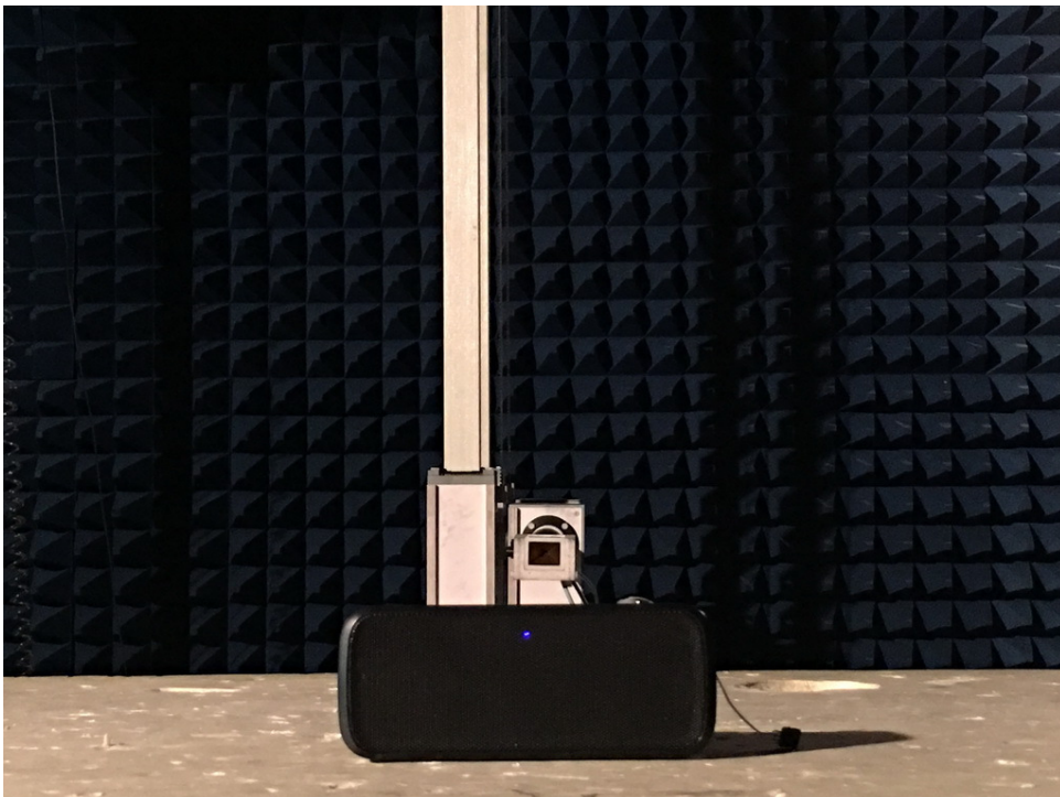
Photograph 4: Set-up for Spurious Emissions (18GHz-26GHz)
