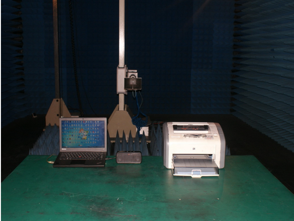
Photograph 7: Set-up for Radiated Emissions, above 1GHz
