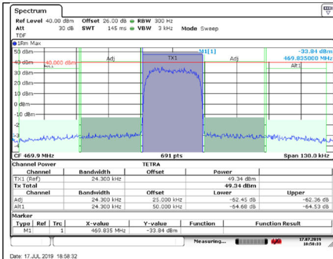
Figure 6.4-31: ACP, Tx @high channel of 460 MHz band, 25 W 0.35TETRA modulation
