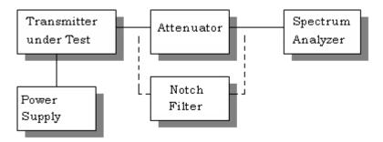
**METHOD OF MEASUREMENT:** The procedure used was ANSI/TIA 603-C: 2004.
