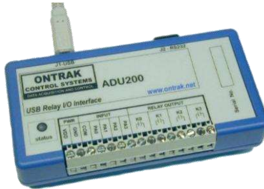
Figure 3-41: Ontrak alarm box
