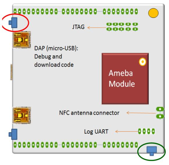
Note: To reset main chip, it is recommended to press Reset button (green-circled) instead of re-plugged in the power cable.
