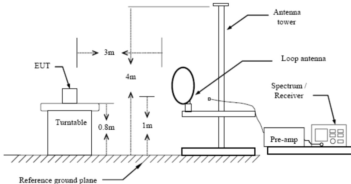
The diagram below shows the test setup that is utilized to make the measurements for emission from 30 MHz to 1 GHz.
