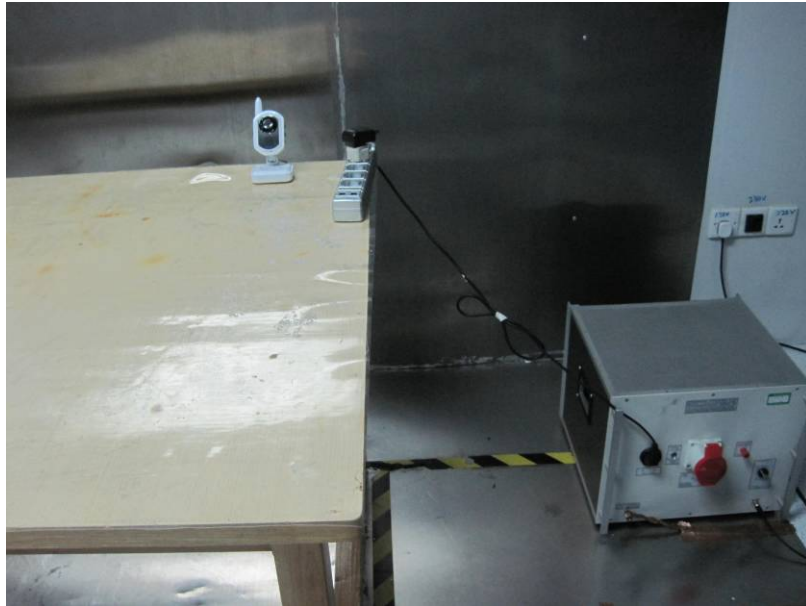
Photograph – Conducted Emission Test Setup
