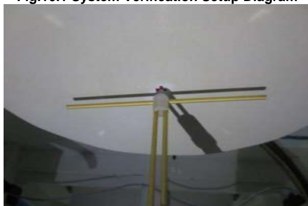
Fig.10.2 Photo of Dipole setup
