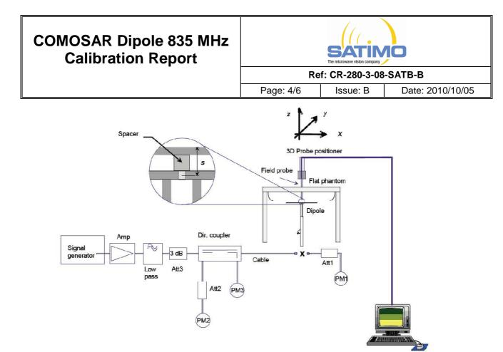
Calibration was performed according to IEEE Std P1528-2003 and OET bulletin 65 Supplement C (Ed. 01-01)
