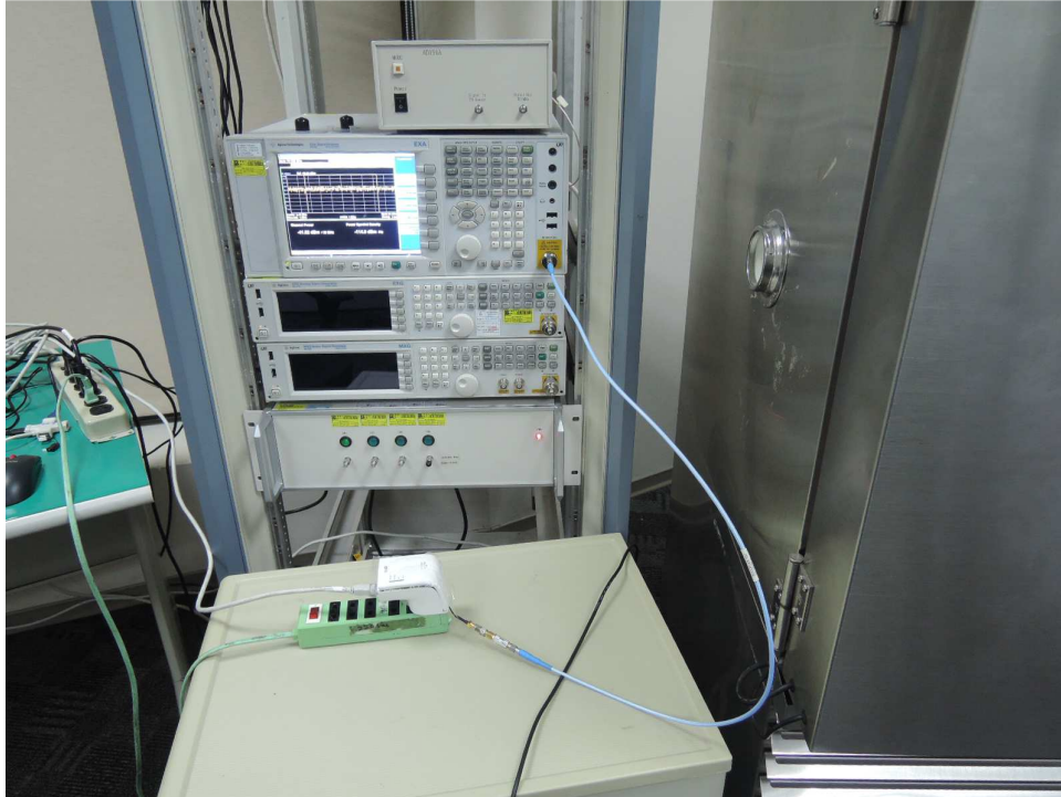
Photograph 4: Set-up for Conducted testing
