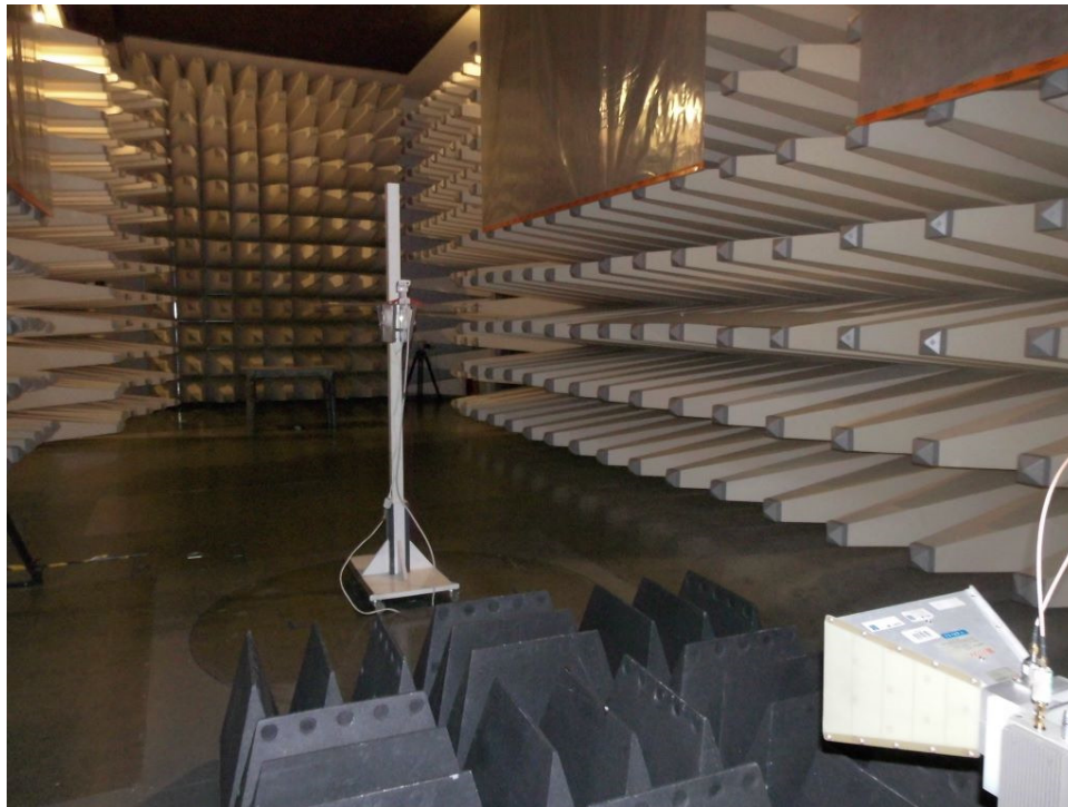
Set-up for Radiated Emission
