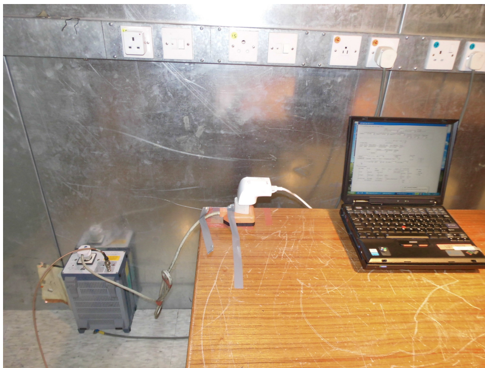
Set-up for AC Mains Conducted Emission
