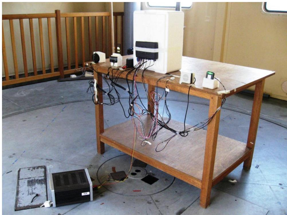
Final measurement, EUT is in horizontal position (right side face to test antenna):
