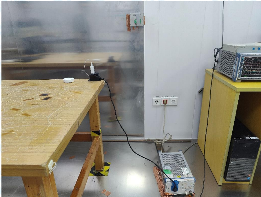
Photo of Setup for Radiated Emission (30MHz~1GHz)
