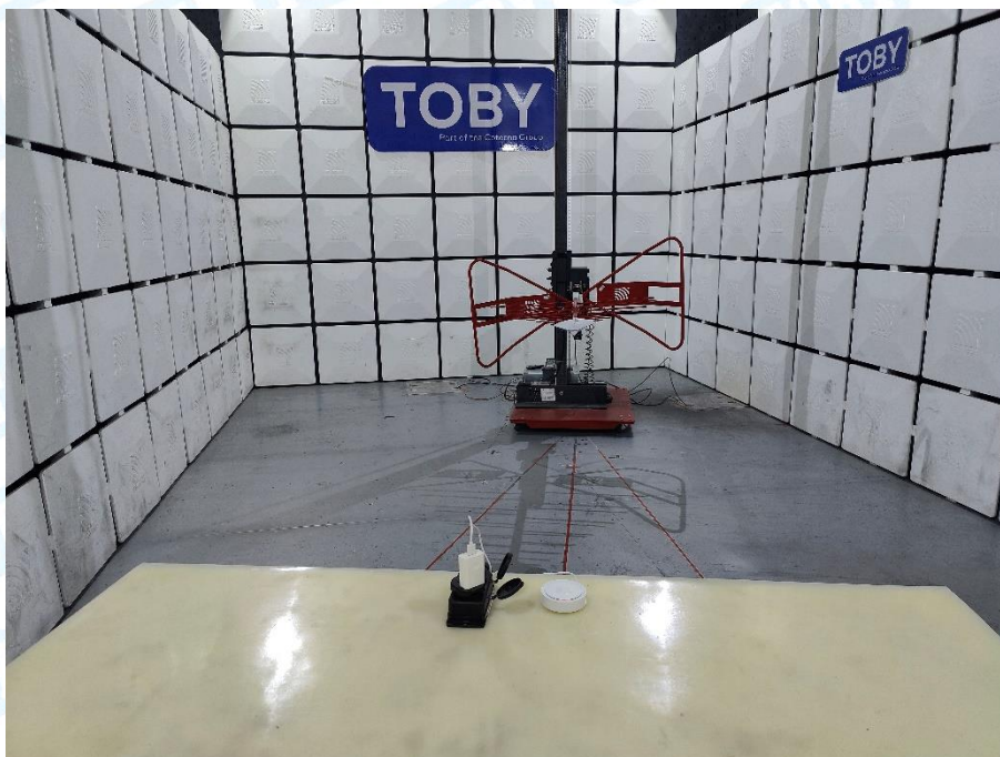
Photo of Setup for Radiated Emission (30MHz~1GHz)
