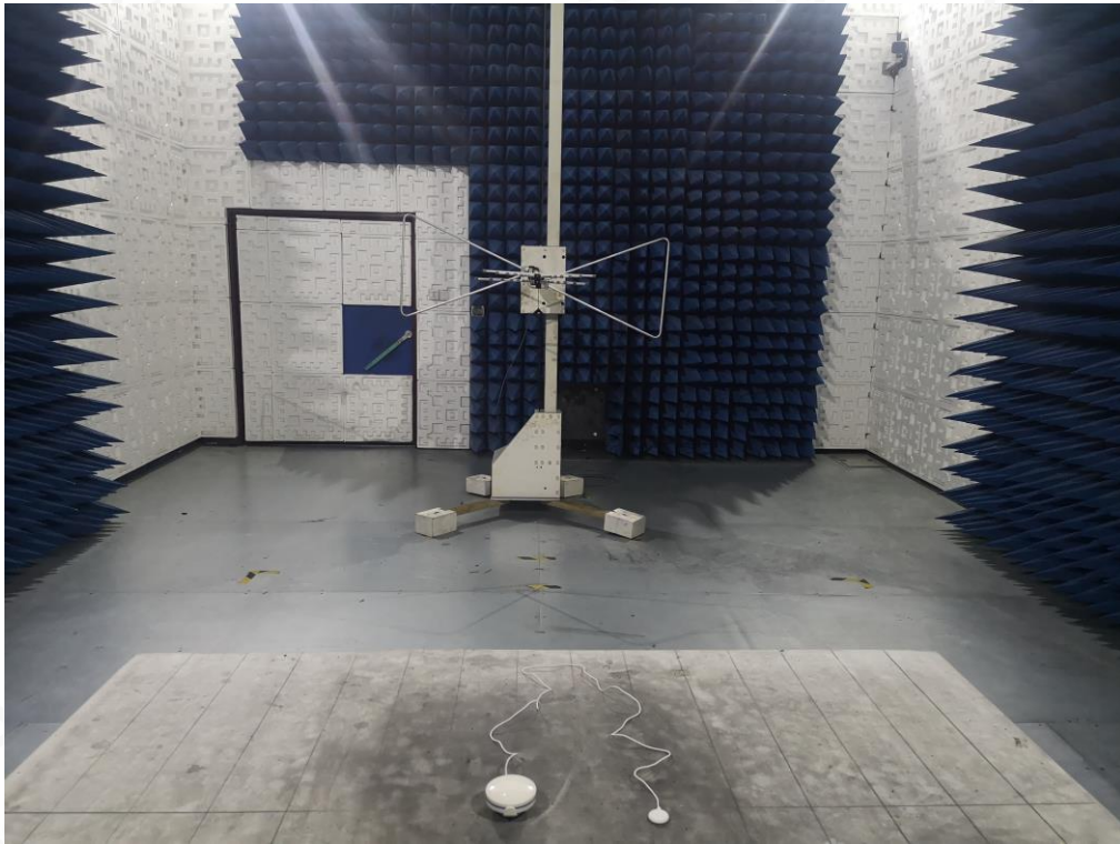
FCC RADIATED EMISSION TEST SETUP ABOVE 1GHZ
