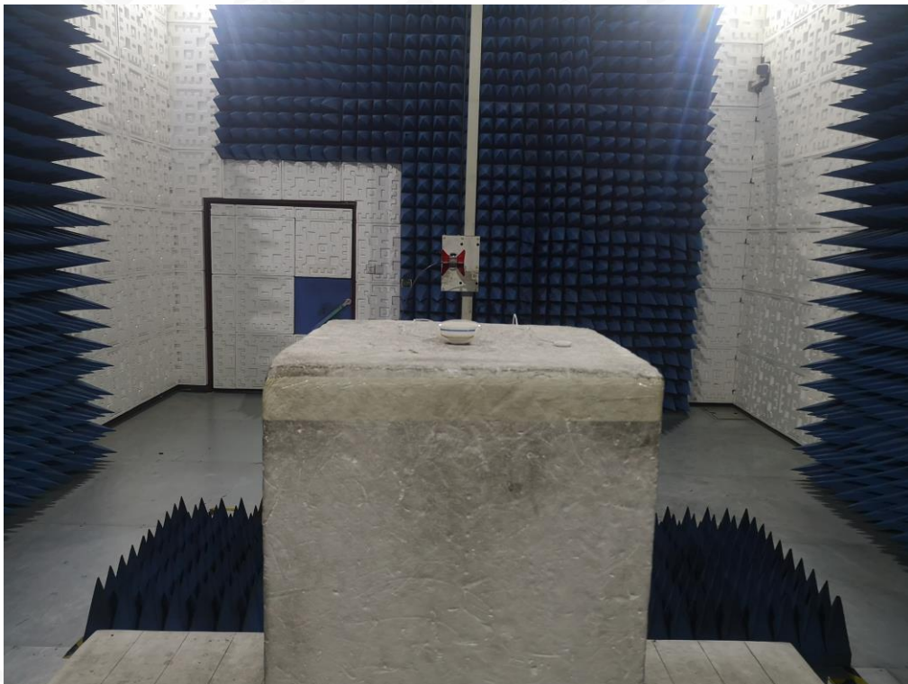
FCC RADIATED EMISSION TEST SETUP ABOVE 1GHZ
