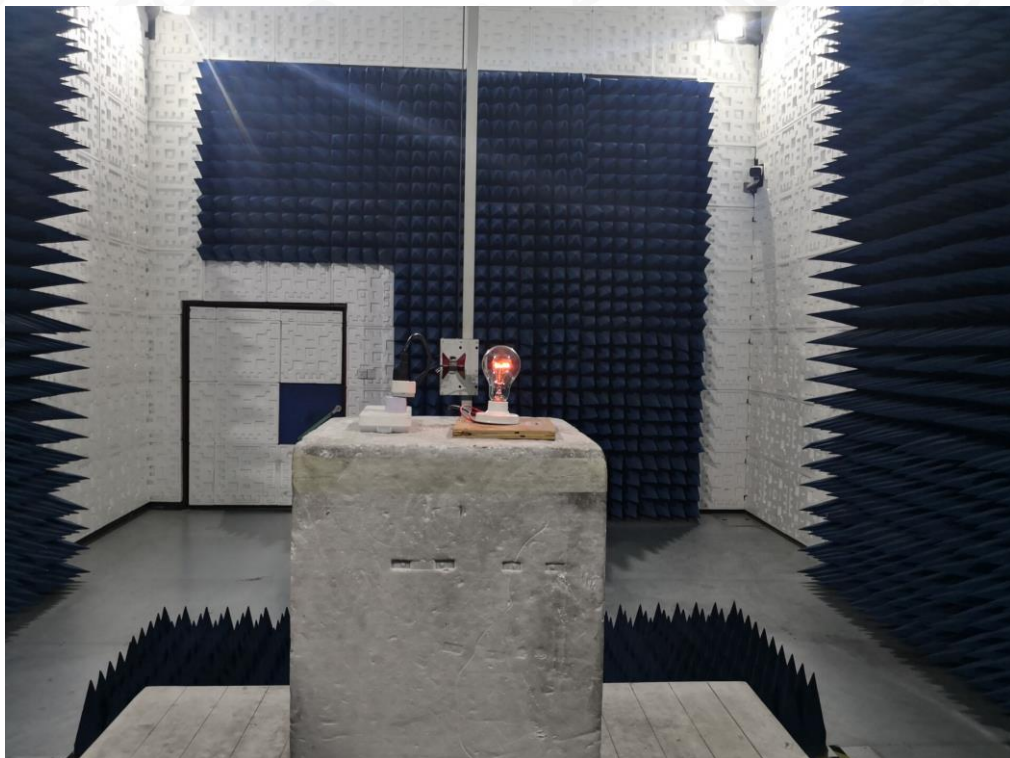
FCC RADIATED EMISSION TEST SETUP ABOVE 1GHZ
