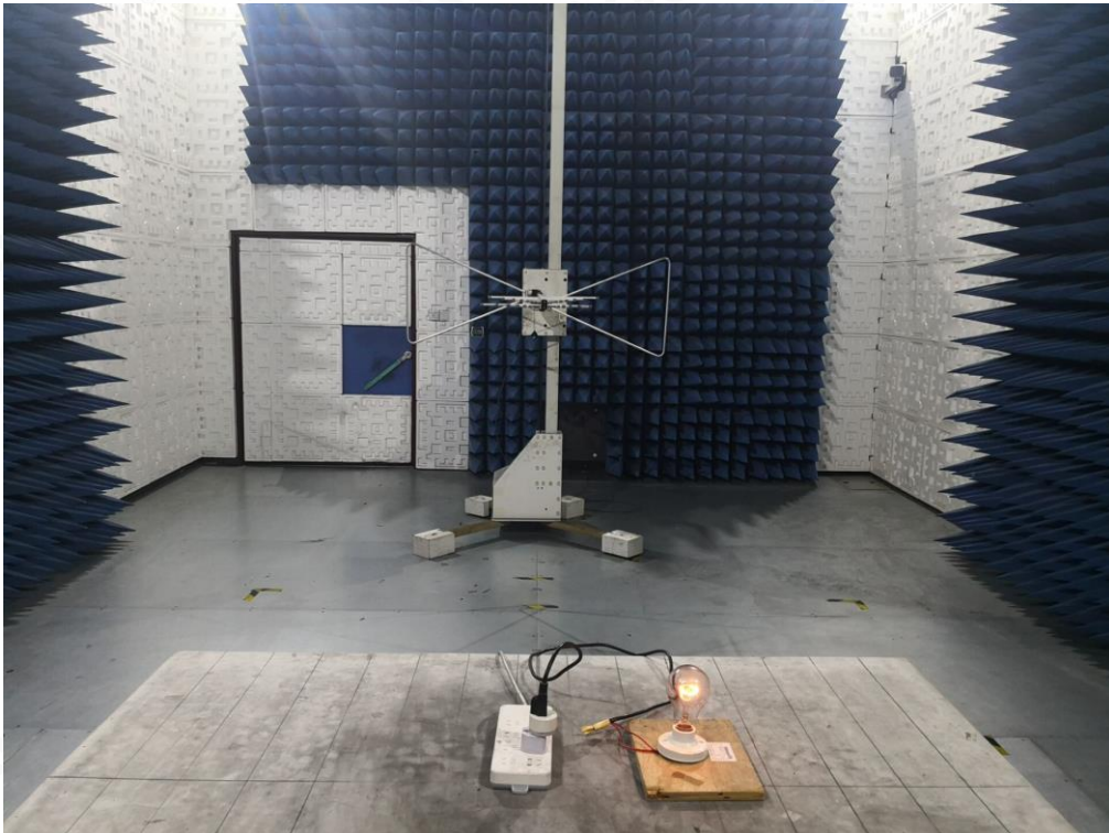
FCC RADIATED EMISSION TEST SETUP ABOVE 1GHZ
