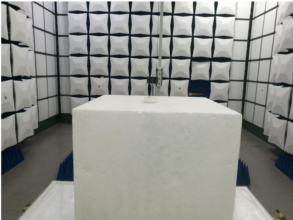
FCC RADIATED EMISSION TEST SETUP ABOVE 1GHZ
