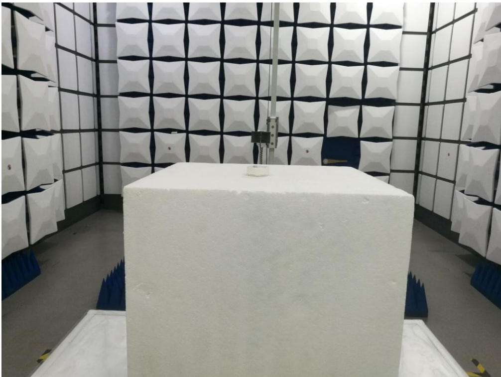
FCC RADIATED EMISSION TEST SETUP ABOVE 1GHZ
