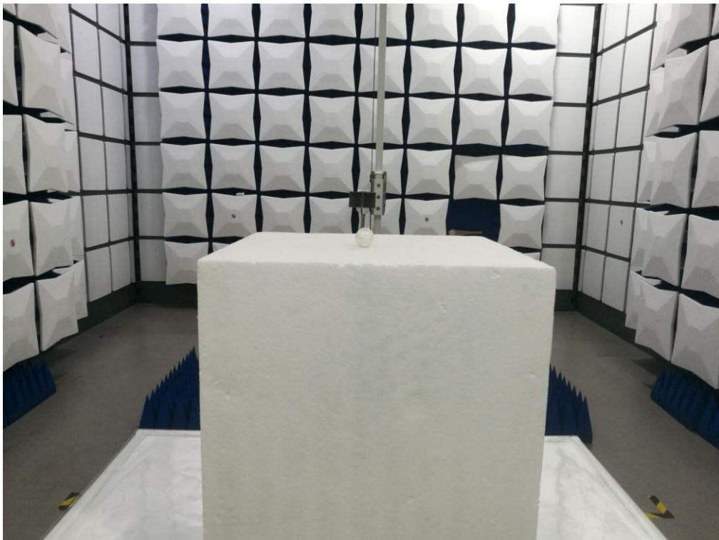
FCC RADIATED EMISSION TEST SETUP ABOVE 1GHZ
