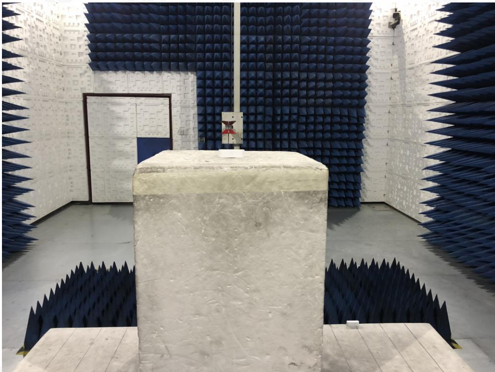
FCC RADIATED EMISSION TEST SETUP ABOVE 1GHZ
