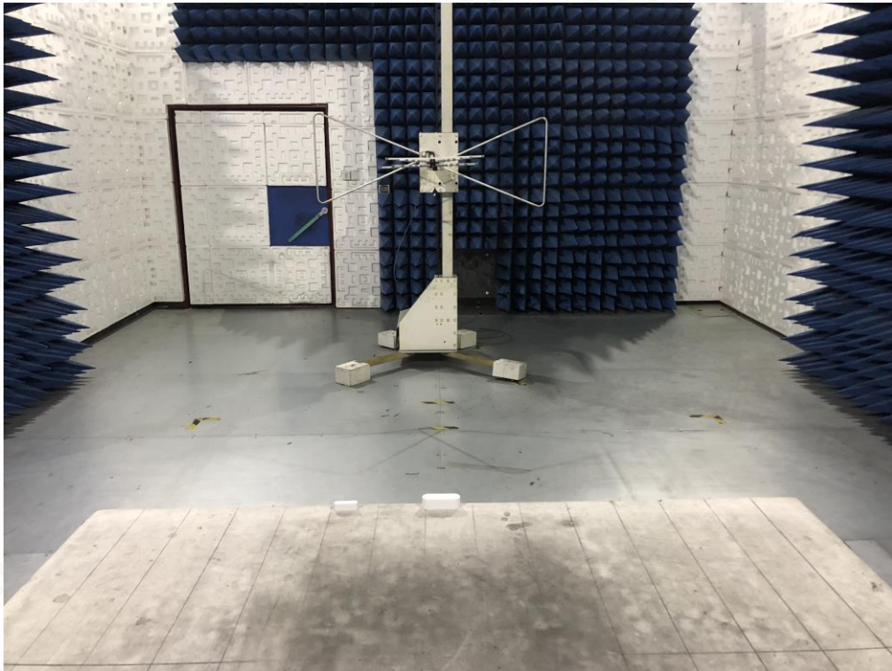
FCC RADIATED EMISSION TEST SETUP ABOVE 1GHZ
