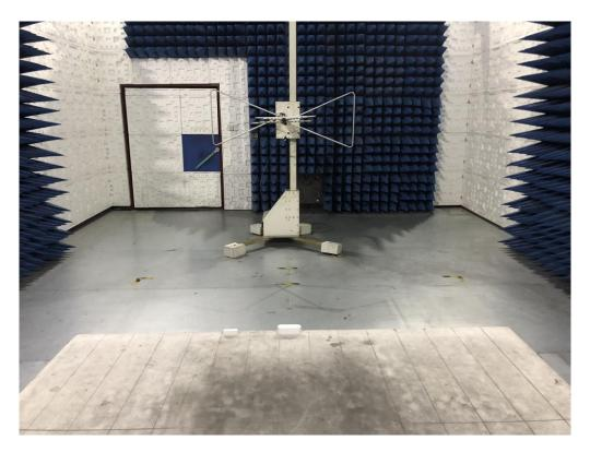
FCC RADIATED EMISSION TEST SETUP ABOVE 1GHZ
