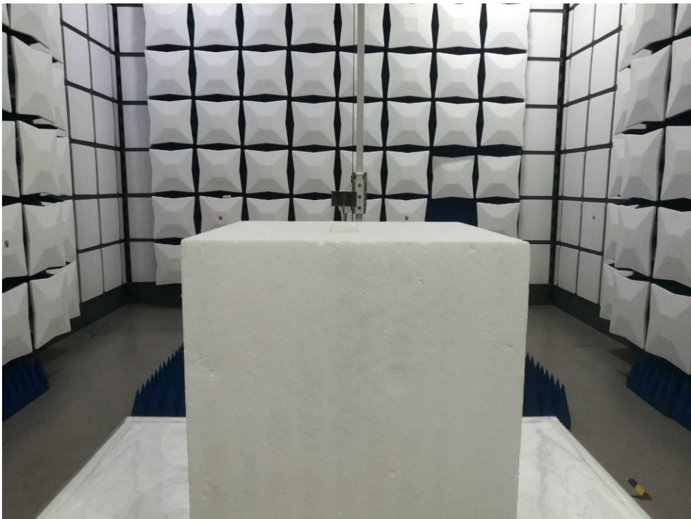
FCC RADIATED EMISSION TEST SETUP ABOVE 1GHZ
