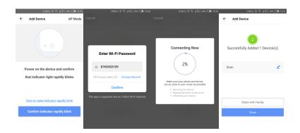
a. In AP mode, press and hold the reset button for 6s after entering the smart WiFi mode. The indicator light will blink slowly.
