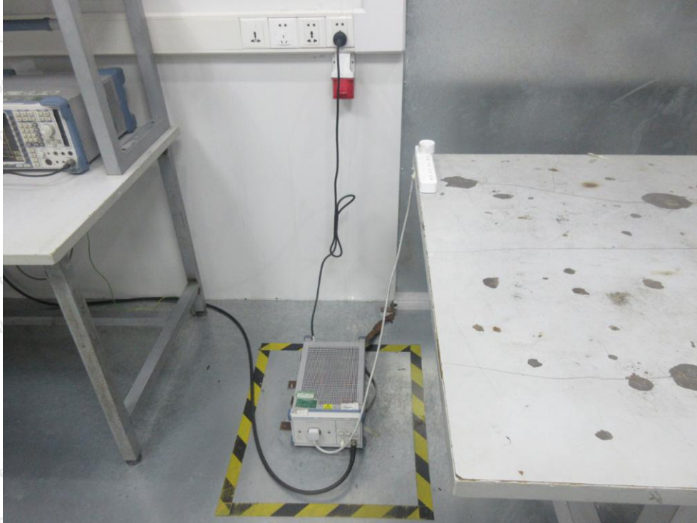
Photo of Conducted Emission Test
