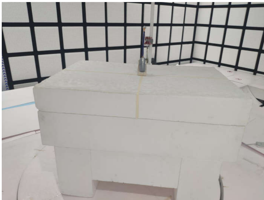
Radiated spurious emission Test Setup-3(Above 1GHz)
