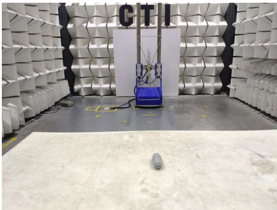
Radiated spurious emission Test Setup-2(Below 1GHz)
