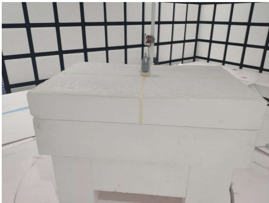
Radiated spurious emission Test Setup-1(Above 1GHz)
