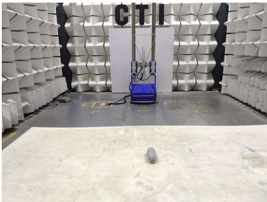
Radiated spurious emission Test Setup-1(Below 1GHz)
