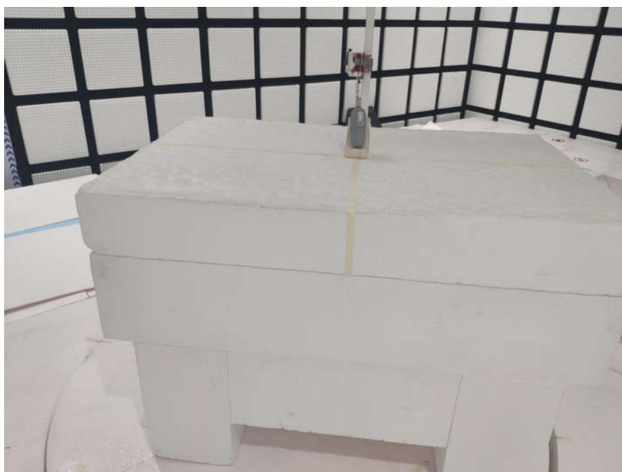
Radiated spurious emission Test Setup-2(Above 1GHz)
