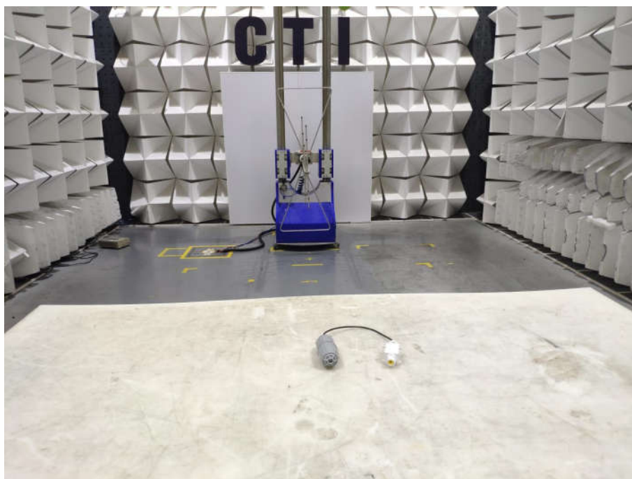
Radiated spurious emission Test Setup-4(Below 1GHz)
