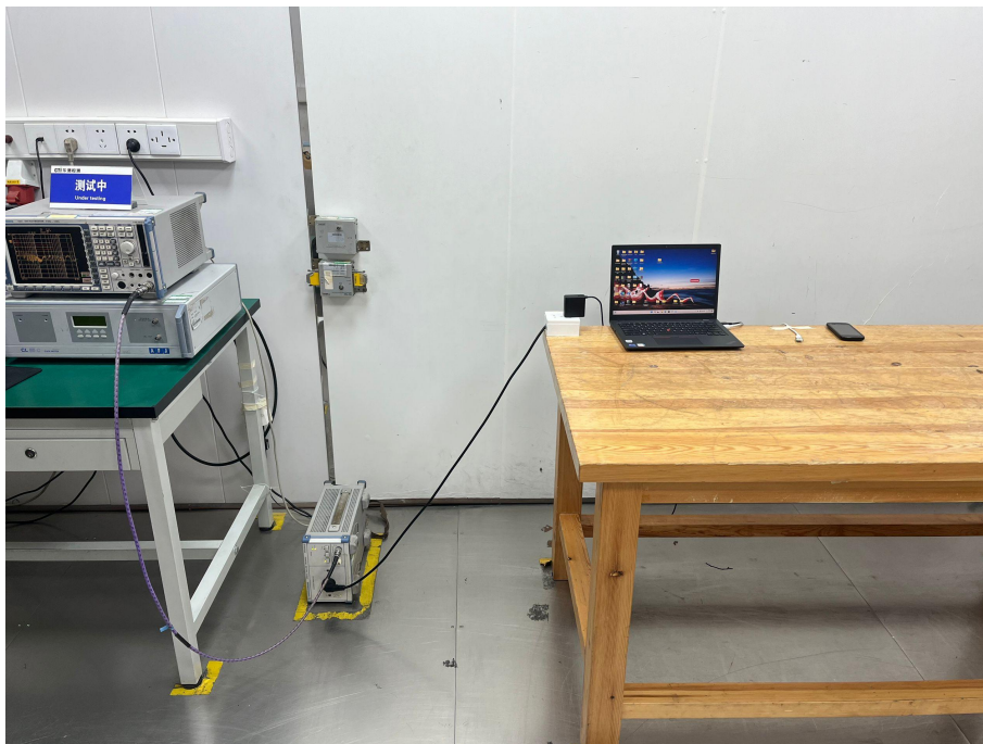
AC Power Line Conducted Emission Test Setup
