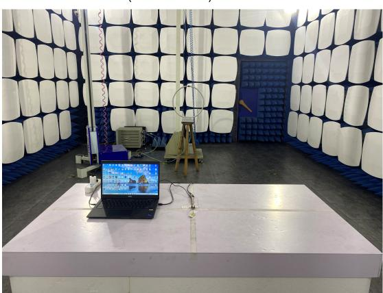
3. Radiated emission (9KHz-30MHz)
