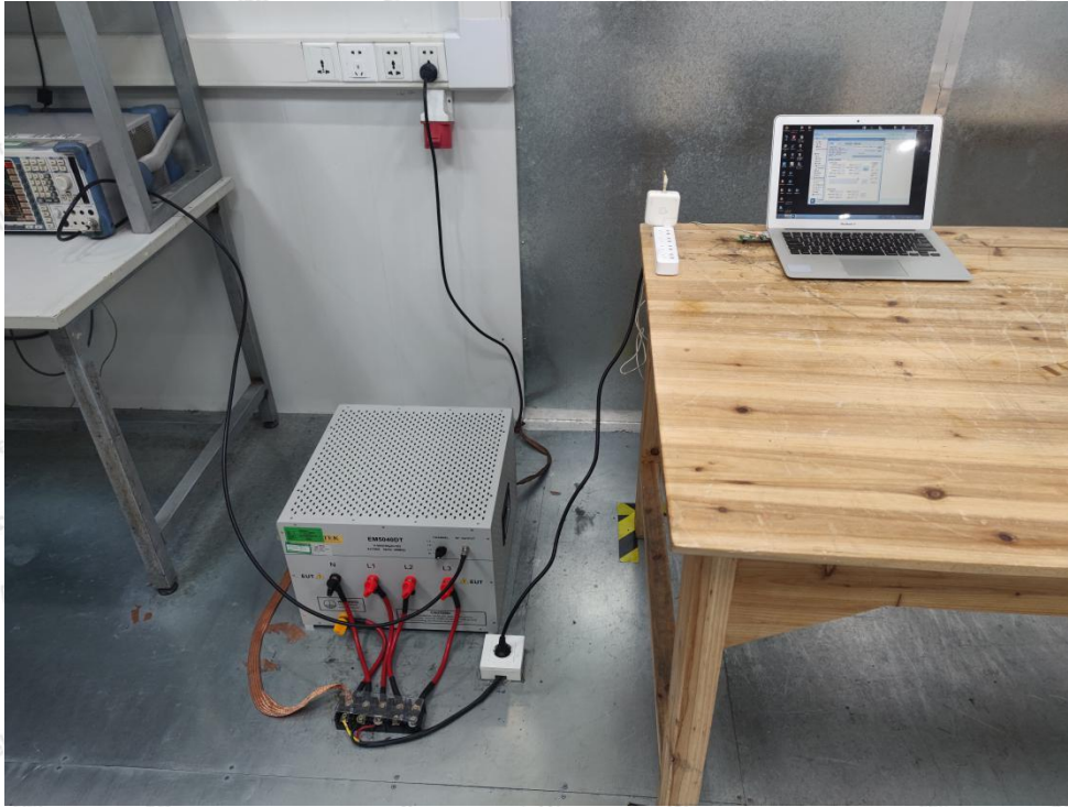
Photo of Conducted Emission Measurement
