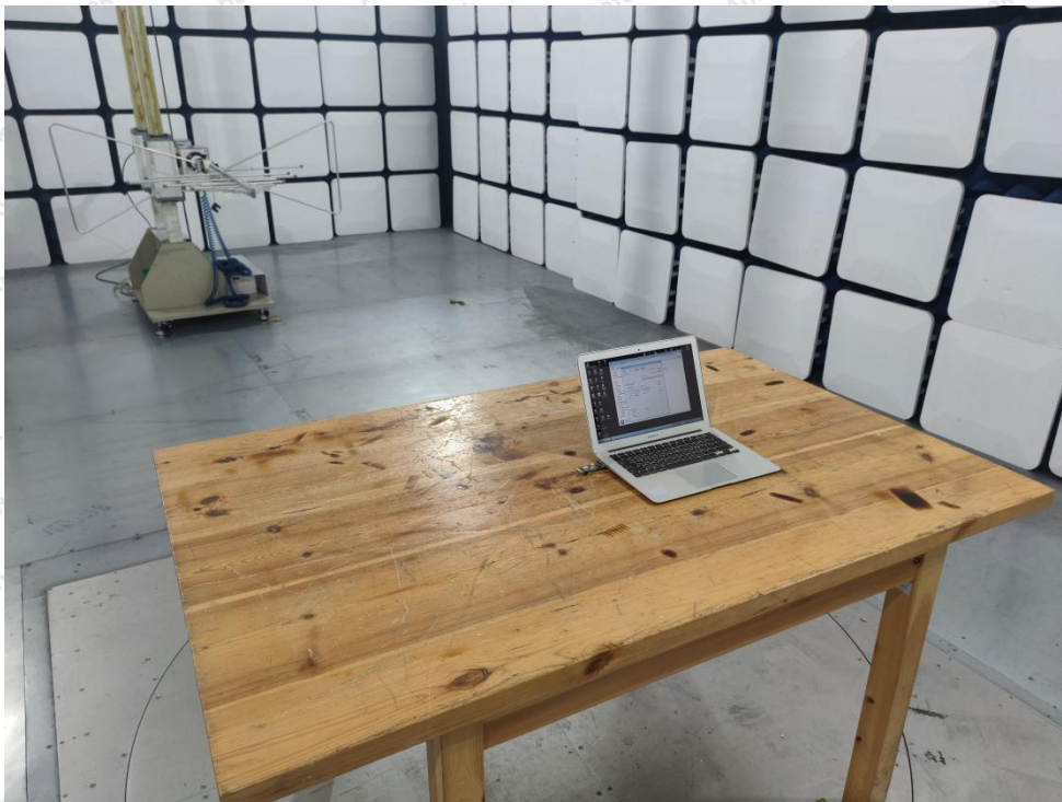
Photo of Radiation Emission Test
