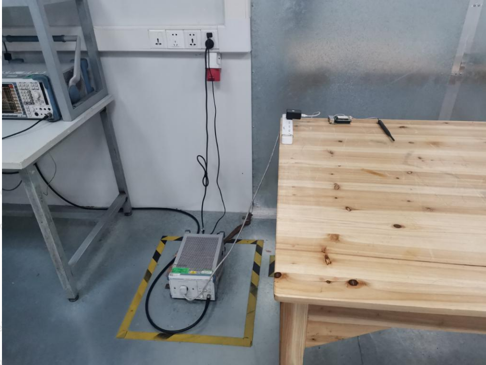
Photo of Conducted Emission Measurement
