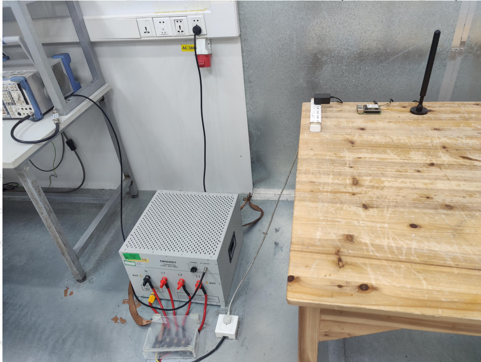
Photo of Conducted Emission Measurement (Sucker antenna)
