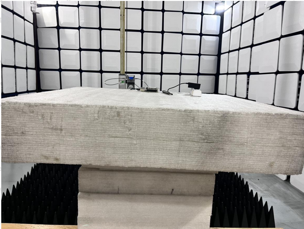
Photo of Radiation Emission Test (Sucker antenna)
