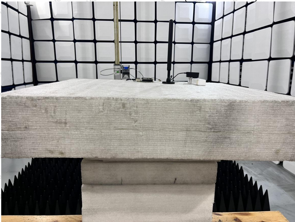
Photo of Radiation Emission Test (Sucker antenna)
