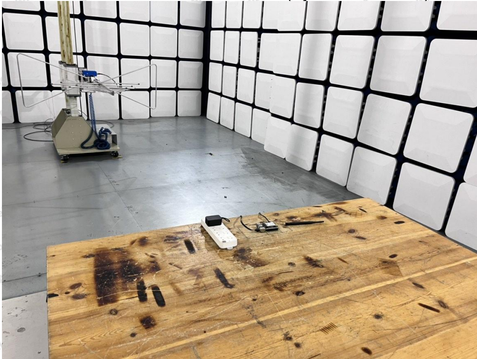
Photo of Radiation Emission Test (Cylindrical antenna)
