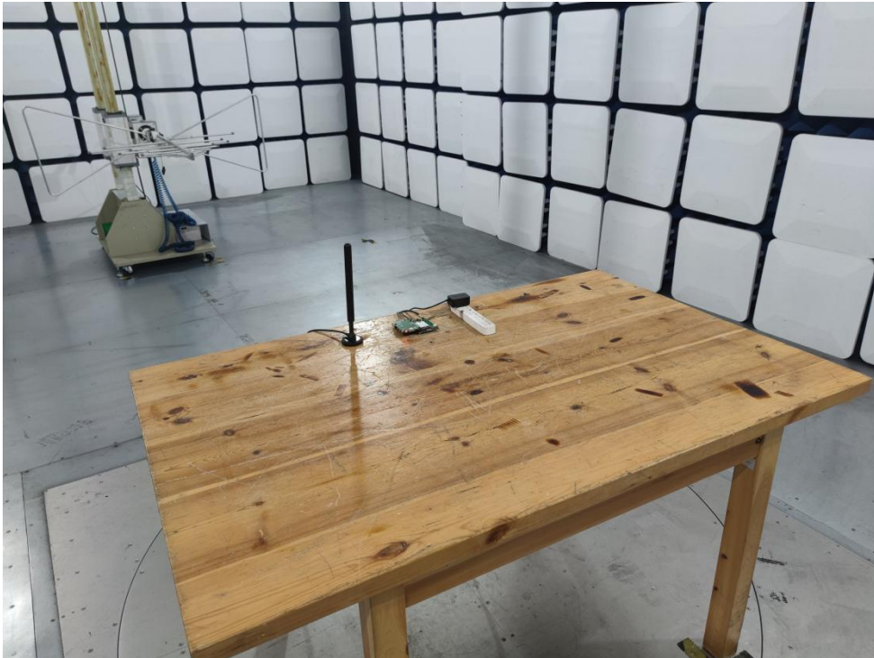
Photo of Radiation Emission Test
