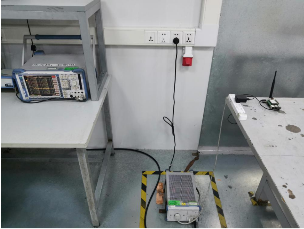
Photo of Conducted Emission Measurement
