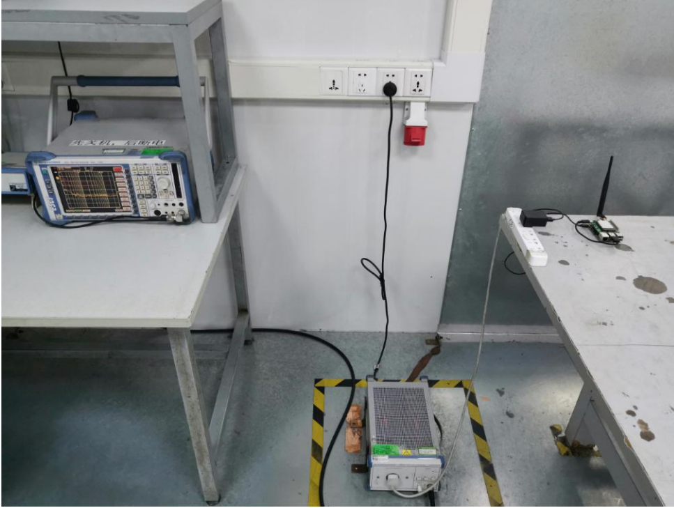
Photo of Conducted Emission Measurement
