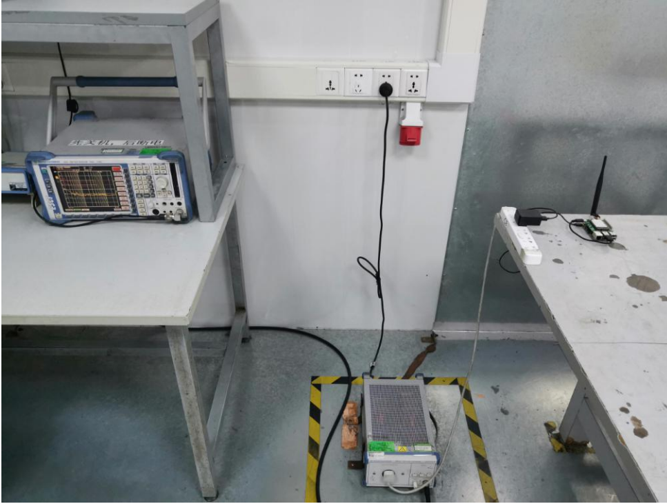
Photo of Conducted Emission Measurement
