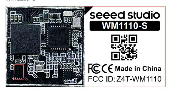
WM1110 has two models , the only difference between this two models is WM1110-S with encryption chip and WM1110-A not.
