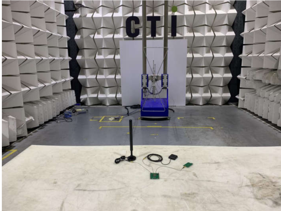
Radiated spurious emission Test Setup-1(Below 1GHz)
